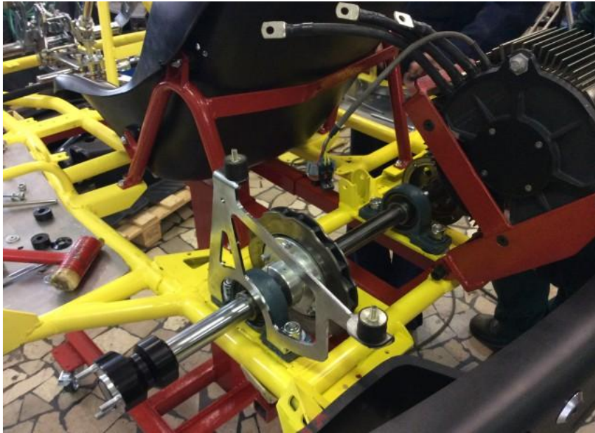
Transmission detail (seen from the right: on the foreground the sprocket for the thermic engine)
