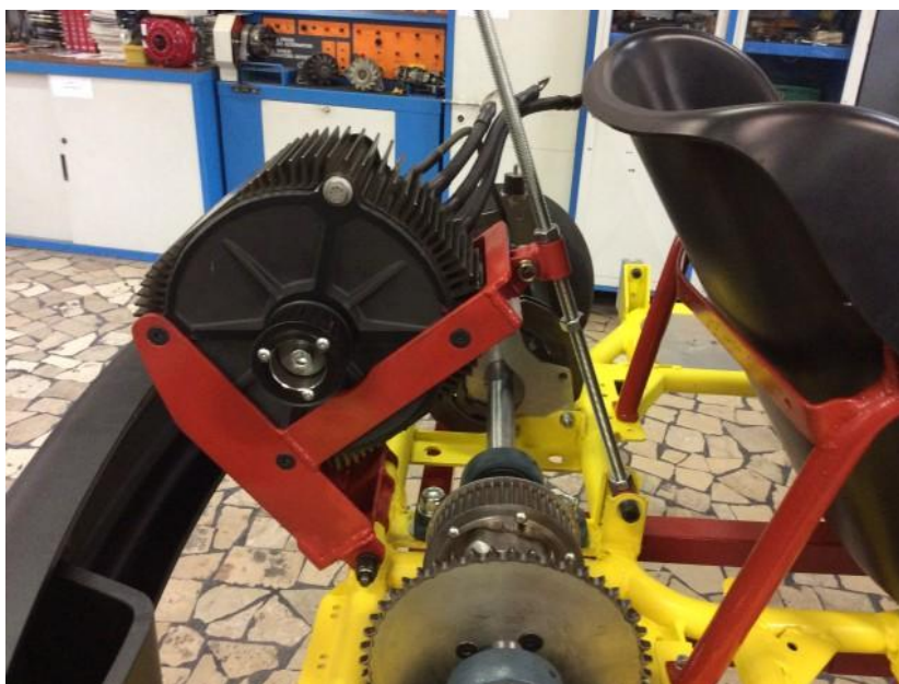
Transmission detail (seen from the right: on the foreground the sprocket for the thermic engine)
