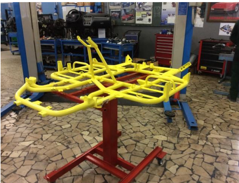
Details of the kart after the components removal and the painting in order to let the structure stand out
