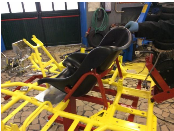
Seat positioned at the centre of the chassis
